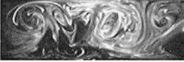
Fig. 6 Instantaneous flow visualization image illuminated over a spanwise-normal light plane located about four pin fin diameters downstream of the pin fin array shown in Fig. 2 for Re_H = 430 ; from Mahmood et al. 24
